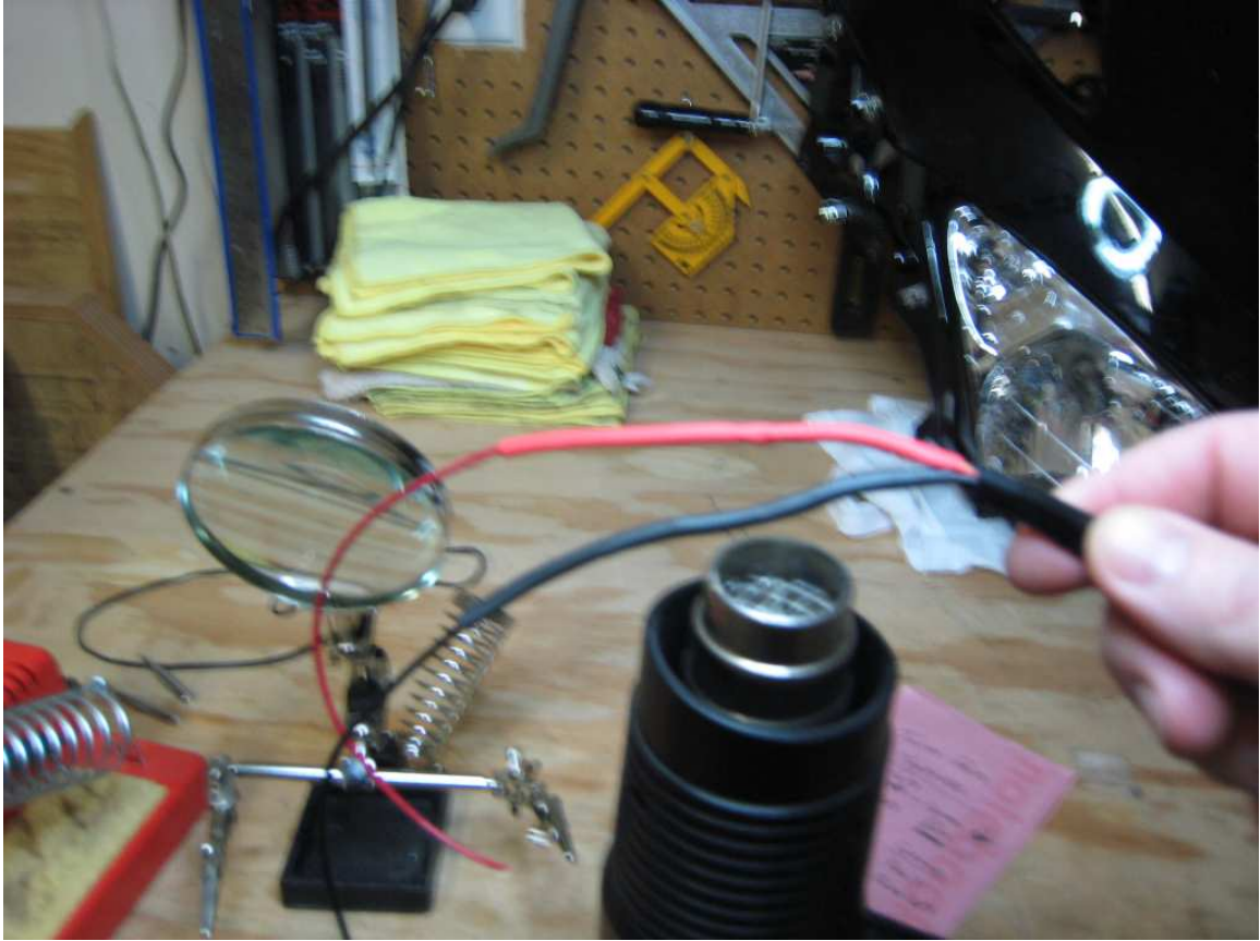
Here we are putting the second layer of shrink tubing on each of the leads.
